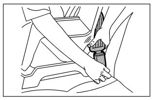
Push the latch plate into the buckle until it clicks. Make sure the release button is positioned so you would be able to unbuckle the safety belt quickly if necessary.
